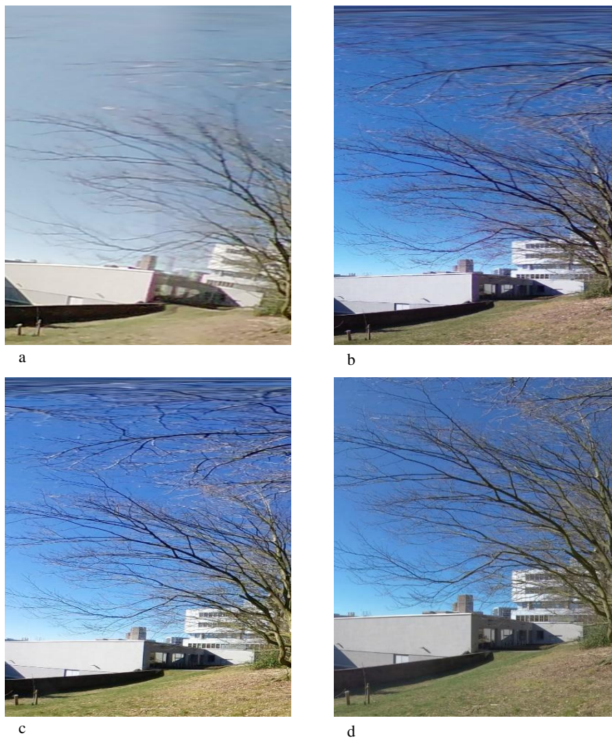
Figure 3. Images with a Zoom Factor recorded with the a 'GoXtreme Omni 360', b 'Ricoh Theta V', c 'Samsung Gear 360' and d 'Insta 360 Pro 2' to compare resolution
