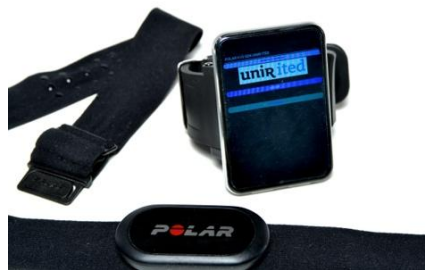
Figure 2. Application Running in a Smartwatch and HRV Wearable Sensor
